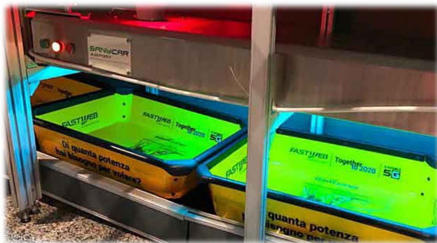
Airport Tray Sanitization, Rome Airport
